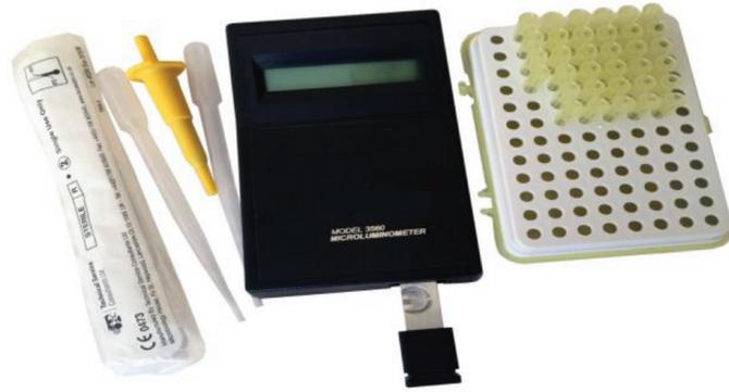
**Figure 3: Profile 1 live bacteria test kit**
